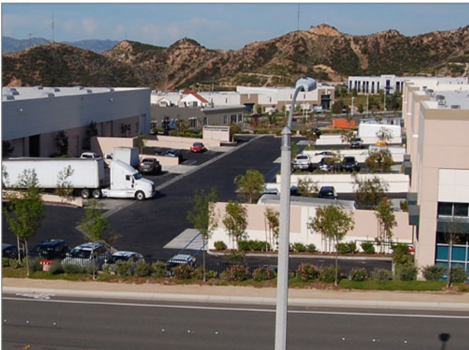
Walls and fences should complement building colors and design. Adjacent plantings should be selected that will grow to soften the wall or fence at maturity.
