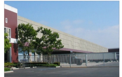
Truck courts should be screened using quality materials on walls or fences.
